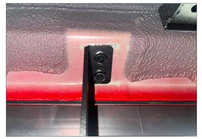
Step 5. Next, tighten the three lower bolts first following with the three upper bolts (15-20 ft./lbs. torque).
